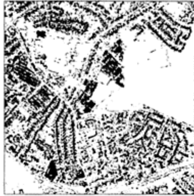
(b) 'built' regions extracted from a land cover classification of a 2m spatial resolution multispectral image of the same area.
