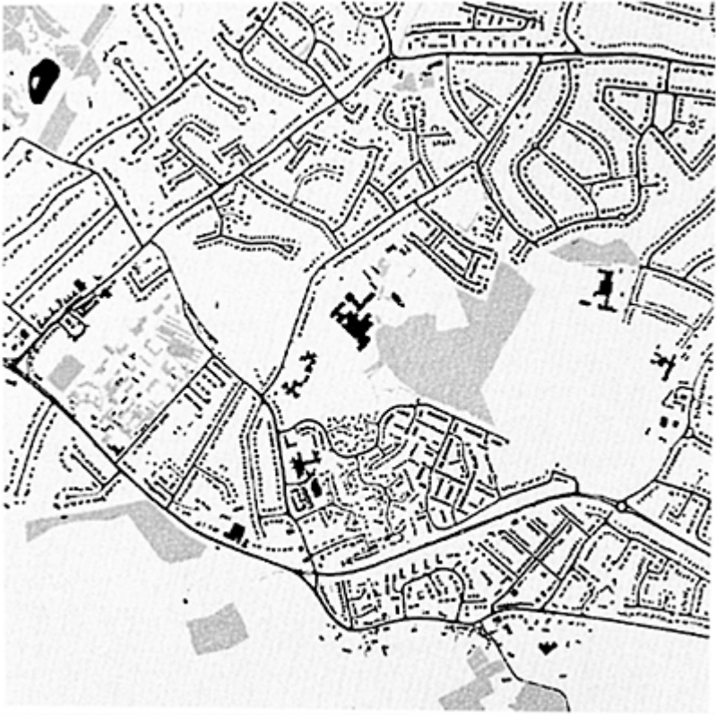
Figure 7.8: Ordnance Survey 1:1,250-scale Land-Line.93+ digital map data covering part of the town of Orpington in the Borough of Bromley, south-east London, U.K. The data have been topologically structured, labelled and converted to a 1m raster.
