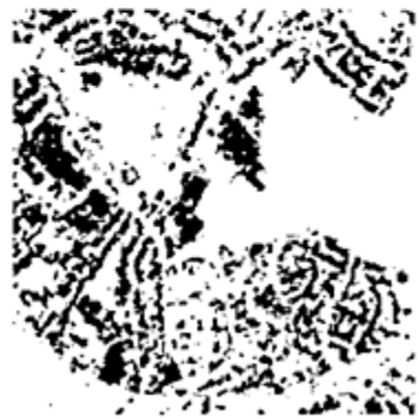
(d) 'built' regions extracted from (b) after applying a conventional, post-classification majority filter using a 3 \times 3 pixel kernel.
