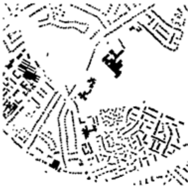
(a) 'built' regions extracted from the 1m spatial resolution land cover map covering part of the town of Orpington in the Borough of Bromley, south-east London, UK.
