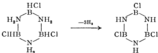
Fig. 125. Dehydrogenation of the hydrochloride of borazole.
