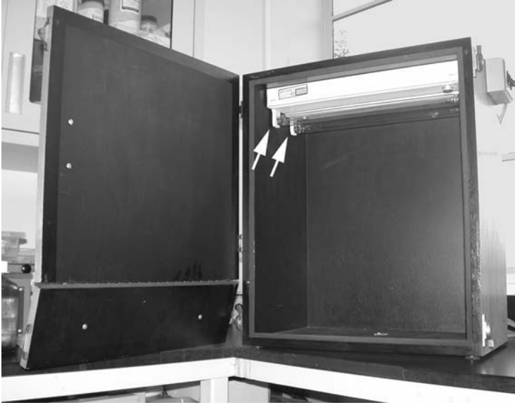
Fig. 1. Typical set up for UV irradiation. The arrows depict the germicidal lamps, which are located in a dark box. Cell culture plates will be placed on a surface for UV irradiation approx 45 cm away from the germicidal lamps.
