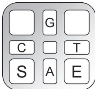
Fig. 4. Enzymes, substrates, and nucleotides are added to the pyrosequencing reaction by the instrument from the PSQ 96 reagent cartridge, where each solution has its specific chamber.
