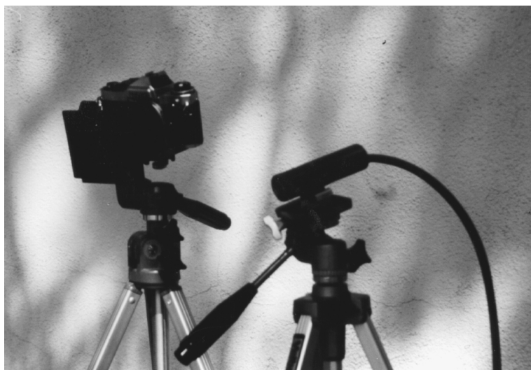
Figure 6.5 Typical tripod-mounted camera and light cable setup for fluorescent-light photography.
