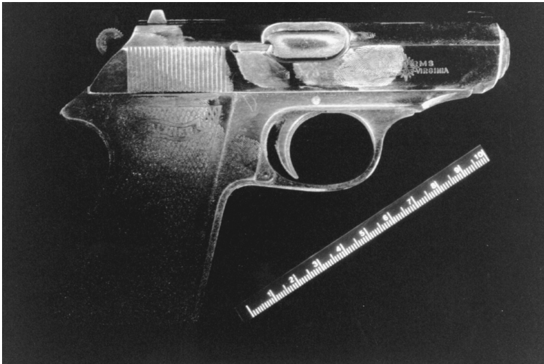
Figure 6.9 Identification and location of latent fingerprint using ALI and red-wop powder. See also color Plate 4 .
