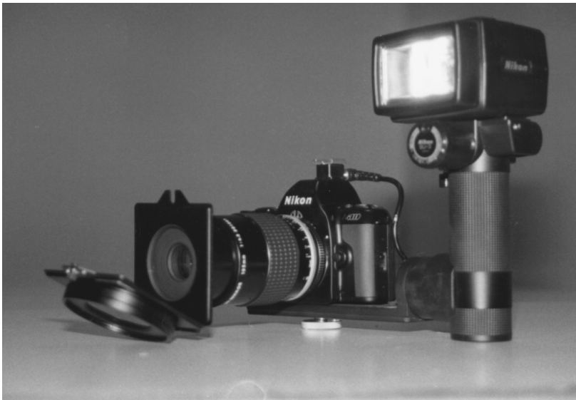
Figure 6.14 Nikon camera setup with Nikon Nikkor UV105 lens, SB140 flash, and Nikon gelatin filter holder AF-1. (Photo courtesy of Nikon, Inc.)
