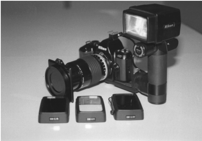
Figure 6.17 Nikon SB140 electronic flash with infrared, visible, and ultraviolet filters.
