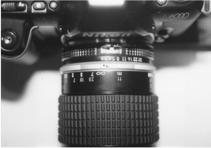
Figure 6.15 Infrared focusing dot on Nikon Nikkor UV105 lens seen as the tiny dot adjacent to the infinity marking on the lens focusing ring. (Photo courtesy of Nikon, Inc.)
