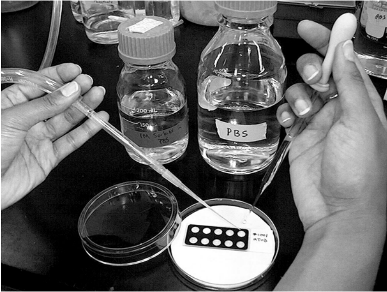
Fig. 3. Washing the slides with PBS. Work quickly so that the wells do not dry out.
