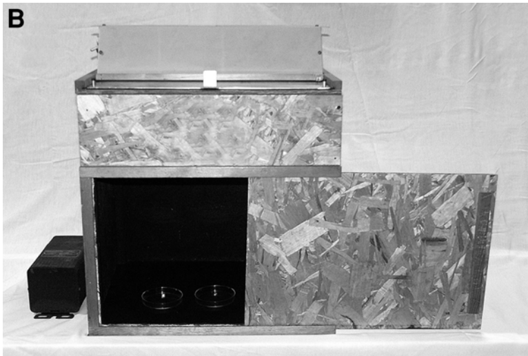
Fig. 1. Source of 254 nm UV light. (A) Photograph of UV light box closed. (B) Same light box opened with Petri dishes inside. (C) ( next page ) Diagram of light box depicting dimensions and side view. Germicidal bulb serving as the source of UV is on top of makeshift shutter system. A voltage stabilizer connecting light fixture to an A/C socket is also presented. The inside walls are painted black, and black material is used for the bottom surface as well. This reduces reflection of light.
