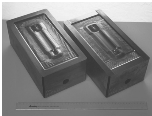
FIGURE 14.42. Precision forging die for the production of turbine blades for aeroengines. 9
