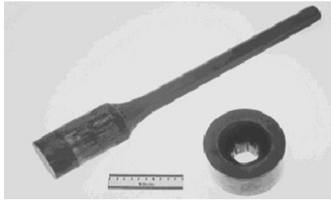
FIGURE 14.41. Extrusion die and as-produced component. 9
