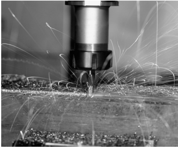
FIGURE 14.38. PVD-coated end mills in a dry high-speed cutting operation.
