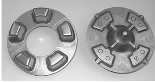
FIGURE 14.43. Moulds for aluminium dye casting.
