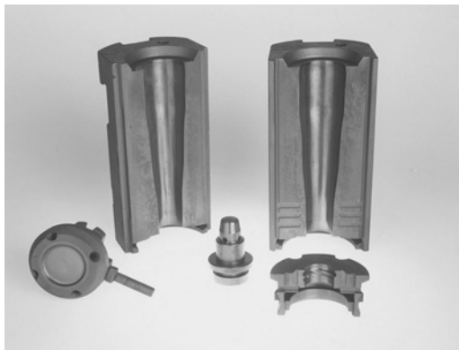
FIGURE 14.40. Coated components for glass-bottle-forming operation. 9
