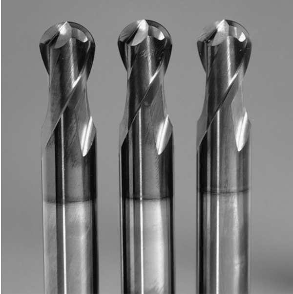
FIGURE 14.54. TiAlYN/VN-coated two-flute ball-nosed cutters (Whisper Mill, Hydra Tools, Sheffield, UK).
