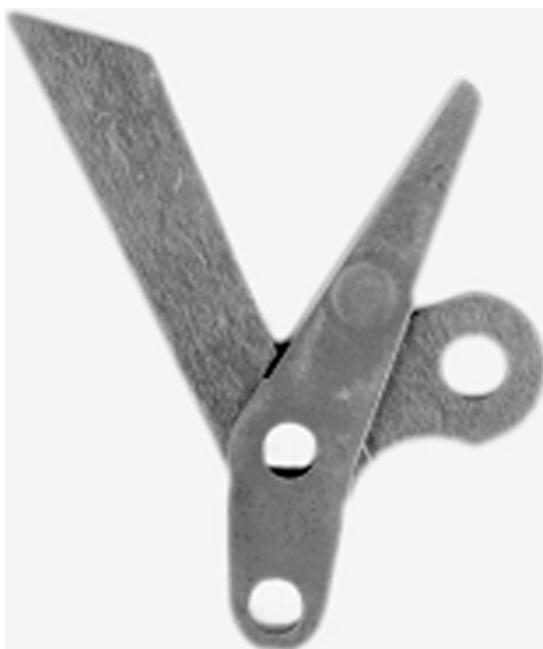
FIGURE 14.78. Textile scissors for cutting various types of textile yarn, coated with low-temperature (250 °C) CrN/NbN superlattice coating. 101
