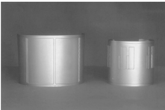
FIGURE 14.85. Label cutting flexible knives coated with low-temperature CrN/NbN superlattice coating.
