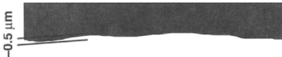
FIGURE 5.9. A plate where the surface is flat but with small long-range fluctuations.
