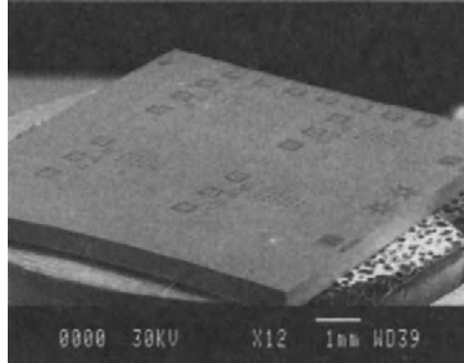
FIGURE 8.3. SEM image of a 1cm 2 patterned Si mold (micron size structures)
