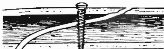
Fig. 8.16 A fully threaded screw inserted in a fully tapped track created while the bones remain apart will have no compression effect on the gap.
