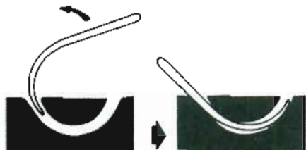
Fig. 4.19 Negotiating a curved channel with a rigid curved dilator. The handle of the dilator must be swung in an arc to direct the point along the curved path.
