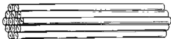
Fig. 4.27 A coherent bundle of glass fibres. They transmit light in a constant relationship within the fibres throughout the bundle.
