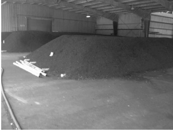
Fig. 13.3 Static pile composting of vegetative and other solid wastes at Joint Base Lewis-McChord, WA
