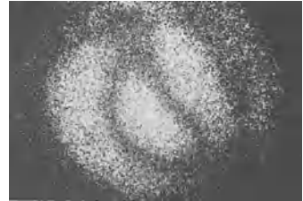
Fig. 4: Double-exposure hologram of the artificial tympanic membrane in the plane scale model of the human outer ear canal (cp. Fig. 2b), recorded with the set-up outlined in Fig. 1, through the special otoscope shown in Fig. 3
