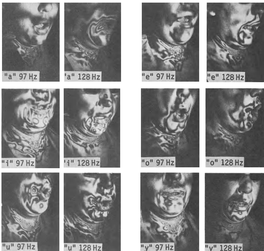
Fig. 4 Holographic interferograms of the vibrations of the frontal part of the neck of a male singing different vowels at two fundamental frequencies 97 Hz and 128 Hz, respectively.
