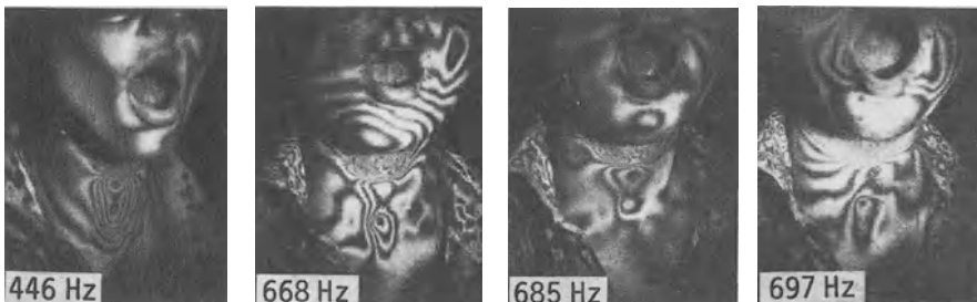
Fig. 3 Holographic interferograms of the vibrations of the frontal part of the neck of a female during singing the vowel "a" at different fundamental frequencies.
