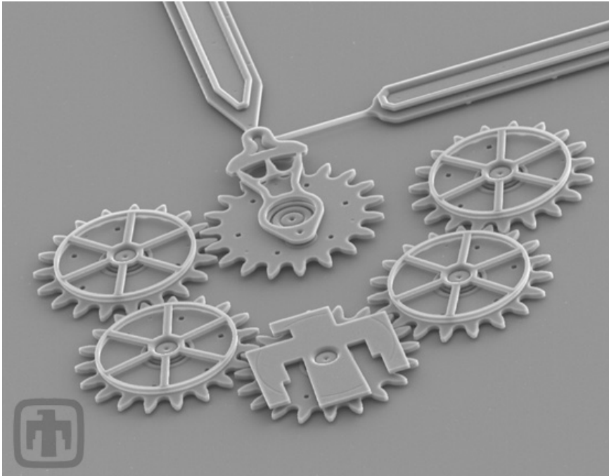
Figure 3.5 An example of micro machine made on silicon substrates. Typical dimensions are several micrometers or smaller. This is a six gear chain. All gears are driven sequentially by the drive gear (top center). Gear chains such as this one have been driven at speeds up to 250,000 RPM. (Courtesy of Sandia National Laboratories, SUMMIT™ Technologies, www.mems.sandia.gov )
