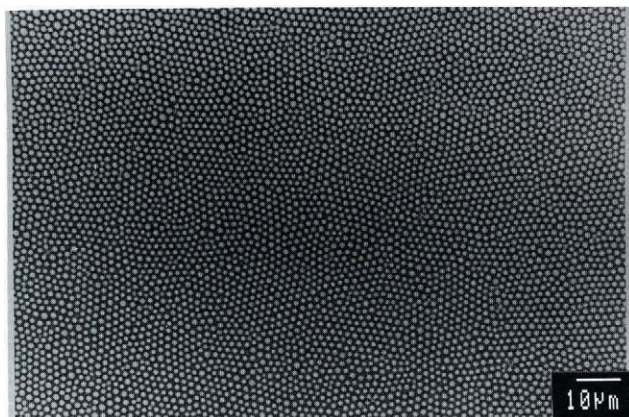
Figure 6. Photomicrograph of O/W emulsion obtained using the SPG emulsification technique (Courtesy of Nakashima and Shimizu 18 )
