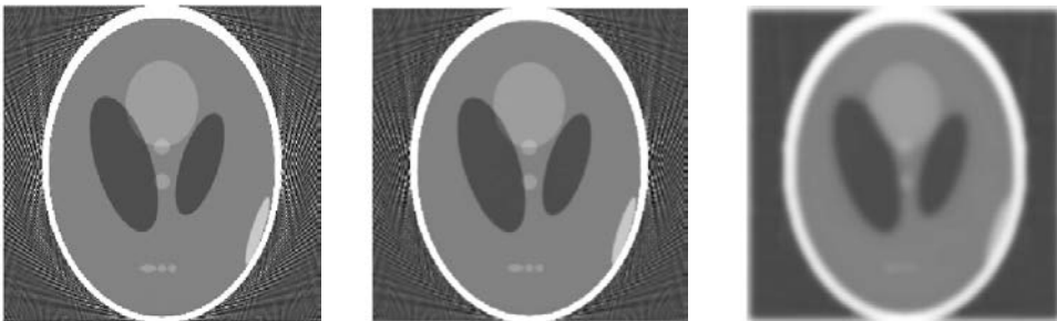
(a) A reconstruction of the Shepp-Logan phantom; see Figure 3.7. (b) The function in (a) convolved with \varphi_\epsilon with a small \epsilon . (c) The function in (a) convolved with \varphi_\epsilon with a large \epsilon .
