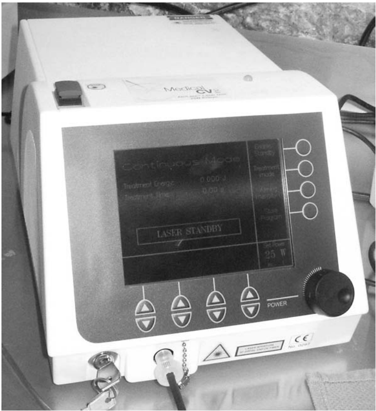
FIGURE 2.4 Photograph of a 25 W continuous wave air-cooled medical diode laser operating at 815 nm.
