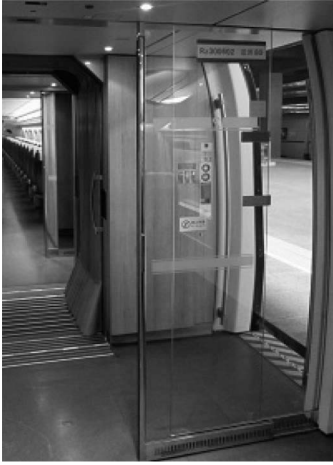
Figure 4. Glass partition and glass door.
