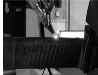
Figure 5. Laser repairing blade of an internal combustion engine.
