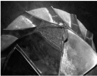
Figure 4. Repair of a turbine impeller.
