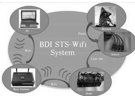
Figure 2. BDI wireless structural testing system equipment components.
