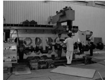
Figure 6. Marine auxiliary engine crankshaft repaired by laser cladding.
