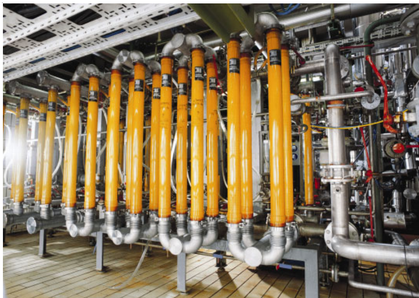
Inlet Figure Enzyme membrane reactor pilot plant at Degussa's research center (Wolfgang, Germany).
