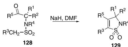
Scheme 34 General synthesis of 2,3-dihydroisothiazole S,S -dioxides: Method G
