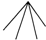
Peak - Formed by four or more lines, when the central vertex is the tallest part of the intersection.
