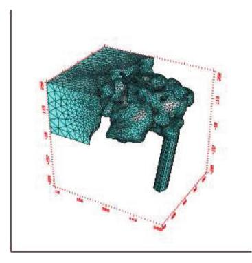
Fig. 2.4 Mesh of a nose and its paranasal sinuses reconstructed from computed tomography with a facial box and a pharyngeal straight distal segment for air flow computations
