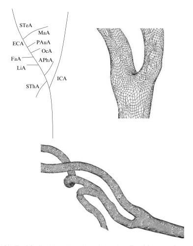
**Fig. 1.24** (**Top left**) Carotid arteries and its main branches. (**Top right**) zoom of a quadrangle surface mesh of the carotid bifurcation suitable for fluid-structure interaction computations using MIT shell element. (**Bottom**) 3DR reconstruction and facetization of the regional artery network
