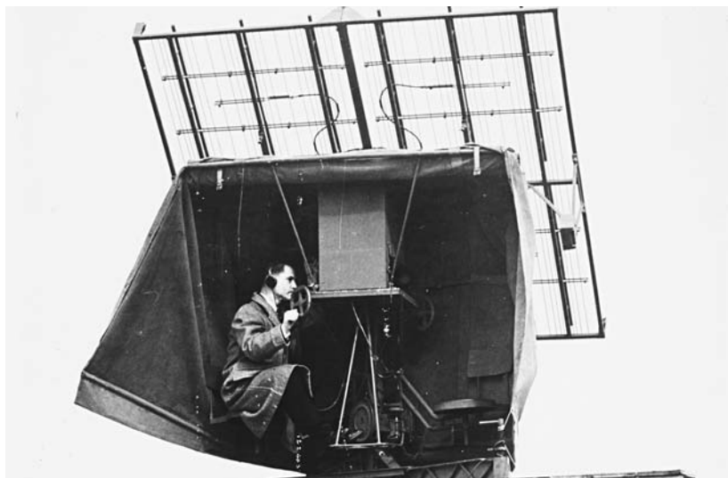
An SCR-658 radio direction finder (“bedspring” antenna) tracks a radiosonde in this photograph from around 1945. (NOAA Photo Library)
