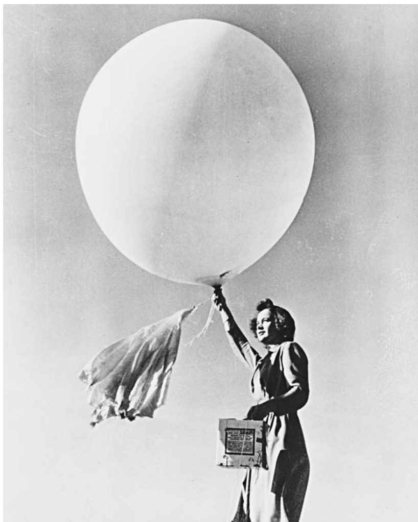
An upper-air observer prepares to launch a radiosonde during World War II. (NOAA Photo Library)
