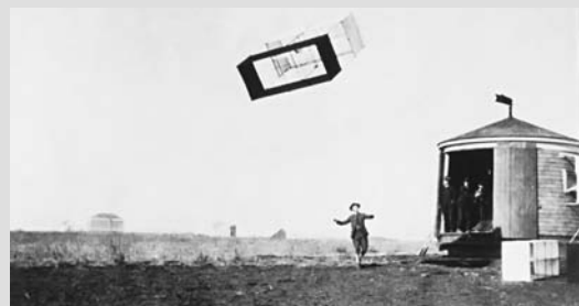
Weather observers launch a large box kite from an early 20th-century aerological observatory. (NOAA Photo Library)
