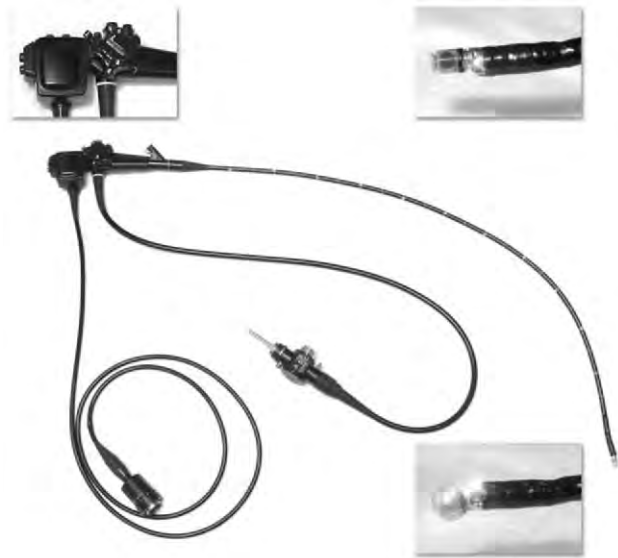
Figure 7-1. The Olympus GF-UM130 ultrasound endoscope. Upper right inset , The control section contains the deflection controls and air/water and suction valves similar to those on a standard endoscope. Upper left inset , The ultrasound transducer is housed in the tip of the endoscope. The forward oblique viewing endoscope and suction channel are proximal to the ultrasound transducer. Lower left inset , The distal tip of the ultrasound endoscope with the water-inflated contact balloon, which covers the ultrasound transducer.
