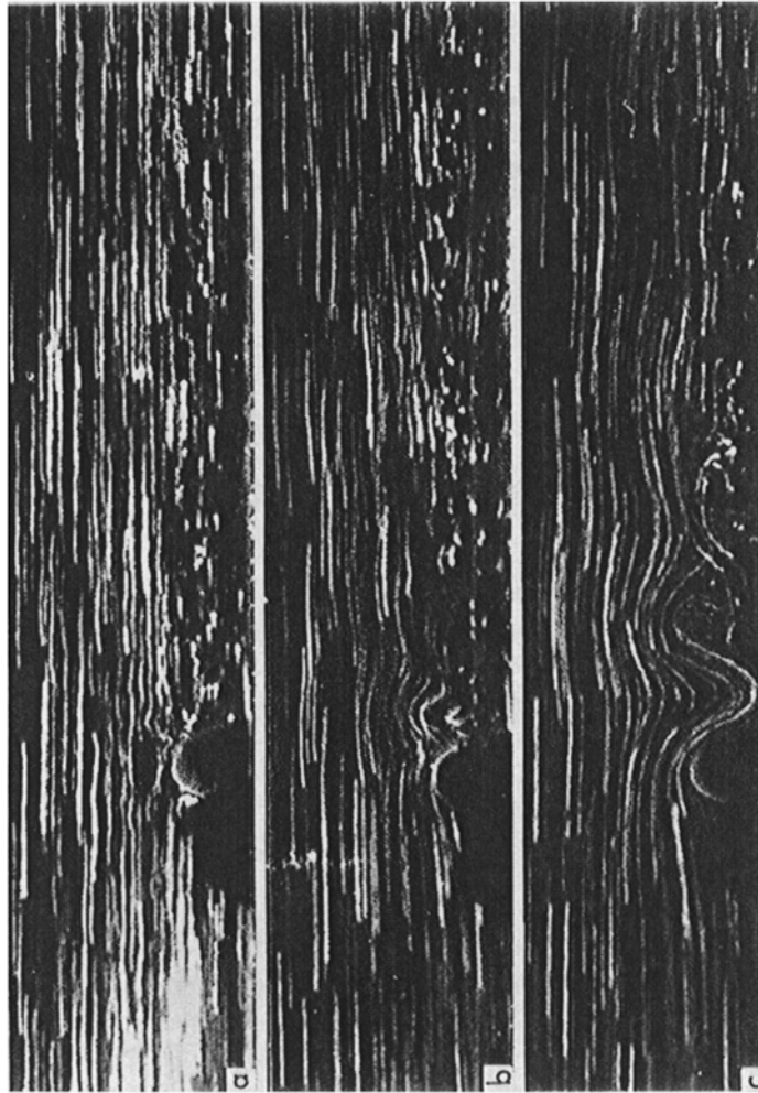
Plate 6 Lee waves developed in simulated northwesterly flow over a model Alpine/Pyrenean topography (courtesy of Professor D.L.Boyer, and the editor and publishers of Meteorology and Atmospheric Physics . From Boyer et al. , 1987). This laboratory experiment is similar to that used in Plate 3. The sequence shows (a) no lee waves, (b) upper level lee waves, and (c) lee waves at all levels, in response to increasing Froude number ( F_0 ). The transitions between cases (a)–(b) and (b)–(c) occur for F_0 \approx 0.25 and 0.37 , respectively; corresponding equivalent atmospheric free stream winds are 8.6 \text{ m s}^{-1} and 12.8 \text{ m s}^{-1} .
