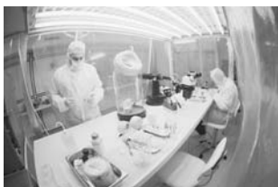
PCBs processing. The production of printed circuit boards requires very clean conditions
