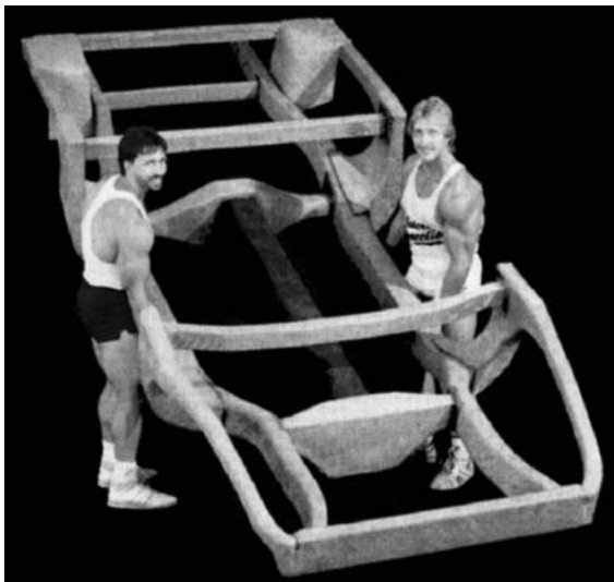
Figure 8.10 An experimental polymeric car frame, based on a graphite–epoxy composite investigated by General Motors to achieve a 60% saving in weight
