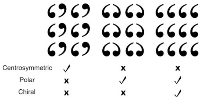
Fig. 9.8 Schematic illustration of centrosymmetric, polar and chiral crystal structures
