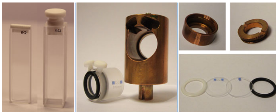
Fig. 6.5 Different types of cuvettes for holding liquid samples. Left: Rectangular type cuvettes, here shown with a pathlength of 1 mm and 1 cm, but shorter types are also available. Middle: A 0.1 mm pathlength round cell with Teflon stoppers shown with a homemade Cu-holder. Right: Demountable round cell (0.1 mm pathlength) consisting of a flat and a hollow quartz plate, shown together with a Teflon and a Viton O-ring (bottom). These may be mounted in the cell holder shown above
