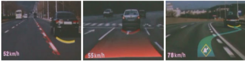
Fig. 3 Augmented reality services on HUD. This shows lane departure warning service, lane curve warning service, and lane change assistance service respectively from the left . These images are captured from our AR-HUD system by placing camera at the position of driver seat
