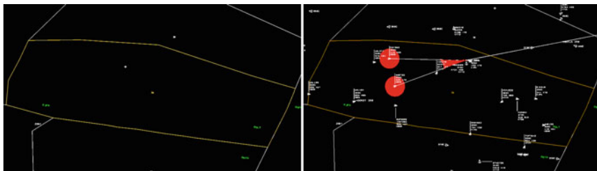
Fig. 1 Screen capture of the controller's radar display in the Conflict Resolution condition before the automation detects a conflict ( left ), and after the automation detects a conflict ( right )
