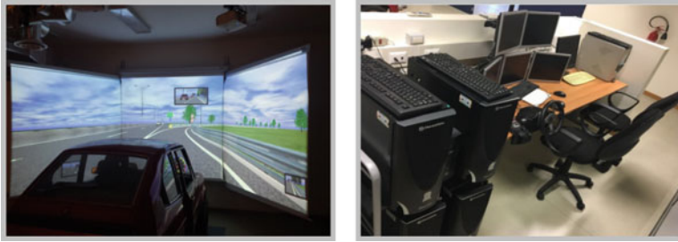
Fig. 1 STISIM driving simulator at the virtual reality laboratory of university research centre for road safety (LASS3)
