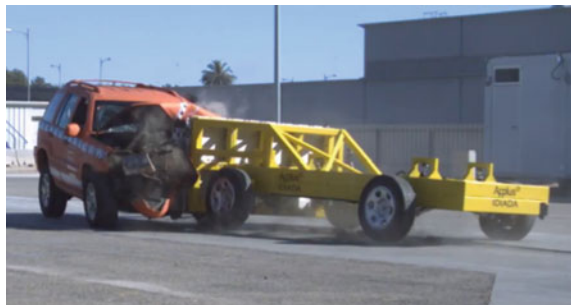
Fig. 12 Image of the RMDB validation test at 77 ms
