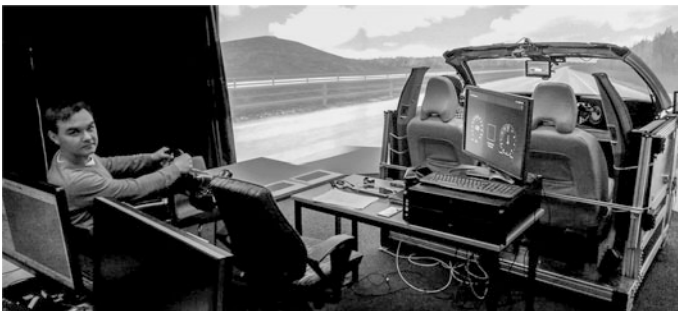
Fig. 4 The driving simulator and the Wizard of Oz driver who acted as the vehicle automation
