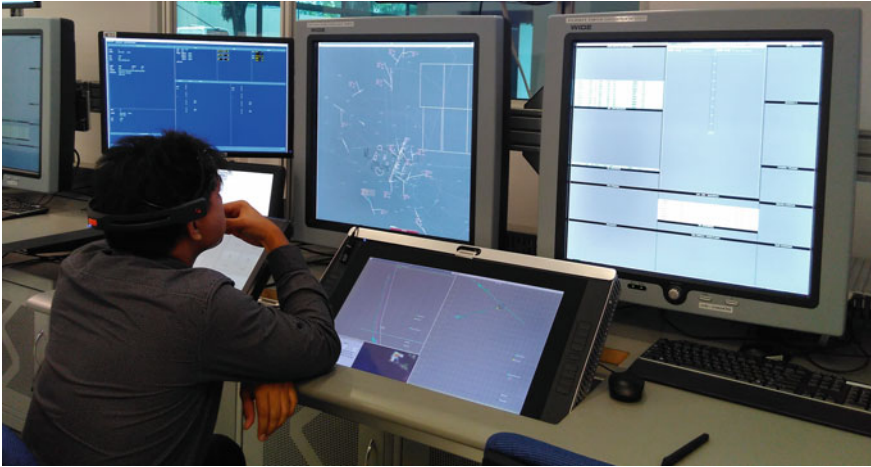
Fig. 6 The air traffic control work place integrated with interactive touch display and brain computer interface
