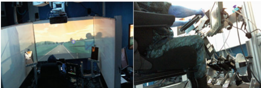
Fig. 5 Display setup of the driving simulator. Left Overhead camera. Right Driving controls and automation display
