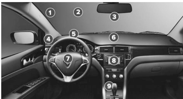
Fig. 2 Proposed locations of mounted mobile phone
