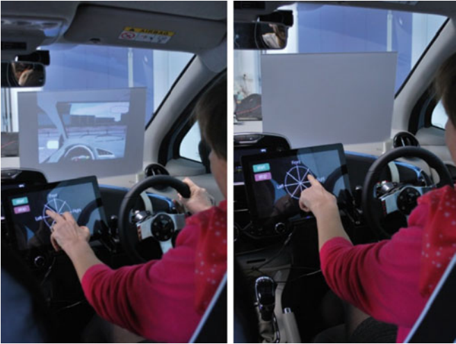
Fig. 2 Experimental set-up used for the simulated driving task ( left ) and the non-simulated driving task ( right )
