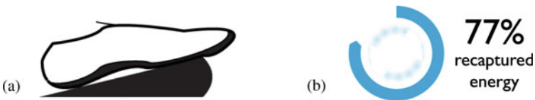
Fig. 6 a Haptic pedal ( left ). Haptic feedback was found in only one on-market vehicle, not available in the US. Pressure exerted by the driver on the throttle is met with corresponding counter-pressure to teach the driver most efficient throttle position during acceleration events. b Regenerative braking feedback ( right ). A display dedicated to regenerative braking feedback depicts total percentage of lost mechanical energy recaptured during a braking event
