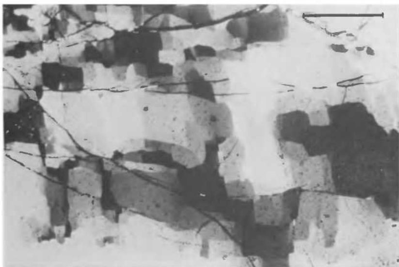
Fig. 6.5. Subgrains in naturally deformed olivine (xenolith from Black Rock Summit, Nevada), optical microscopy, plane-polarized light (scale bar=1 mm) (courtesy J. C. Mercier).
