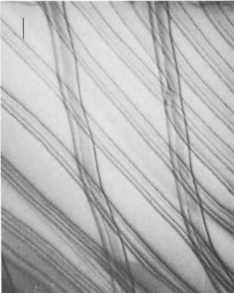
Fig. 2.11. Splitting of dislocations in talc into four partials separated by stacking-fault ribbons. Transmission electron microscopy. Scale bar = 1 \mu\text{m} (courtesy P. Delavignette).
