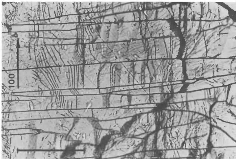
Fig. 6.3. Subgrain boundaries in olivine (xenolith from San Quintin, Baja California, Mexico). Decoration by oxidation. Tilt boundaries in plane (100) (scale bar: 100 \mu\text{m} ) (courtesy J. C. Mercier).
