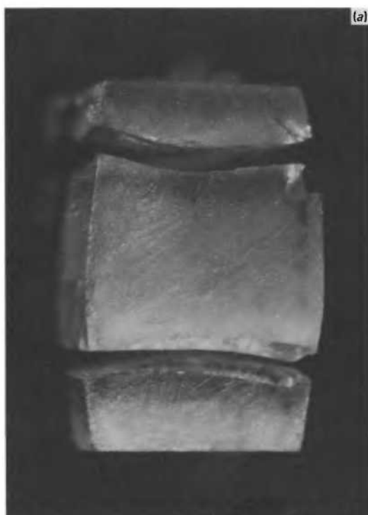
Fig. 1.12. Bending of planes in compressed samples of sodium chloride. Cleavage follows the bent \{100\} planes (not slip planes) normal and parallel to the load axis. Height of sample: top – 8.4 mm; bottom – 5.6 mm (courtesy V. Pontikis).
