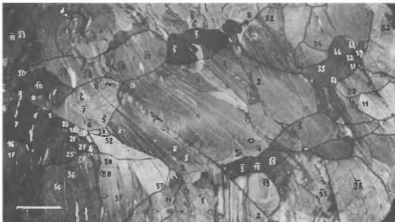
Fig. 6.11. Rotation recrystallization in NaCl single crystal deformed by 70% at T=600^\circ\text{C} and \sigma=40\text{ g/mm}^2 . Etch pits. Subgrains are labelled with their misorientation in degrees with respect to the subgrain 0 (near the centre) 30 denotes a 30^\circ rotation in the counter-clockwise sense and 30 a 30^\circ rotation in the clockwise sense (scale bar=1 mm) (courtesy M. Guillopé).
