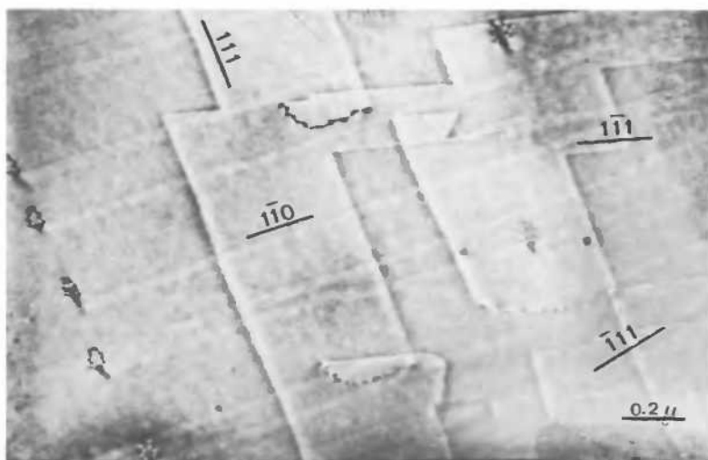
Fig. 4.4. Cross-slip in aluminium. Slip traces in a foil crept in situ in HVEM at 520 °C. TEM at 100 keV (courtesy D. Caillard).
