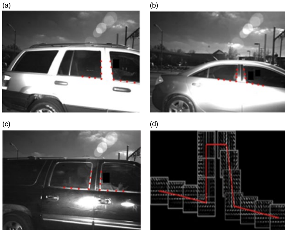
Figure 4.6 Parts (a–c) show a set of landmark points overlaid on three images for B-pillar detection. Part (d) illustrates the spatial shape model for tree structure learned in training.
