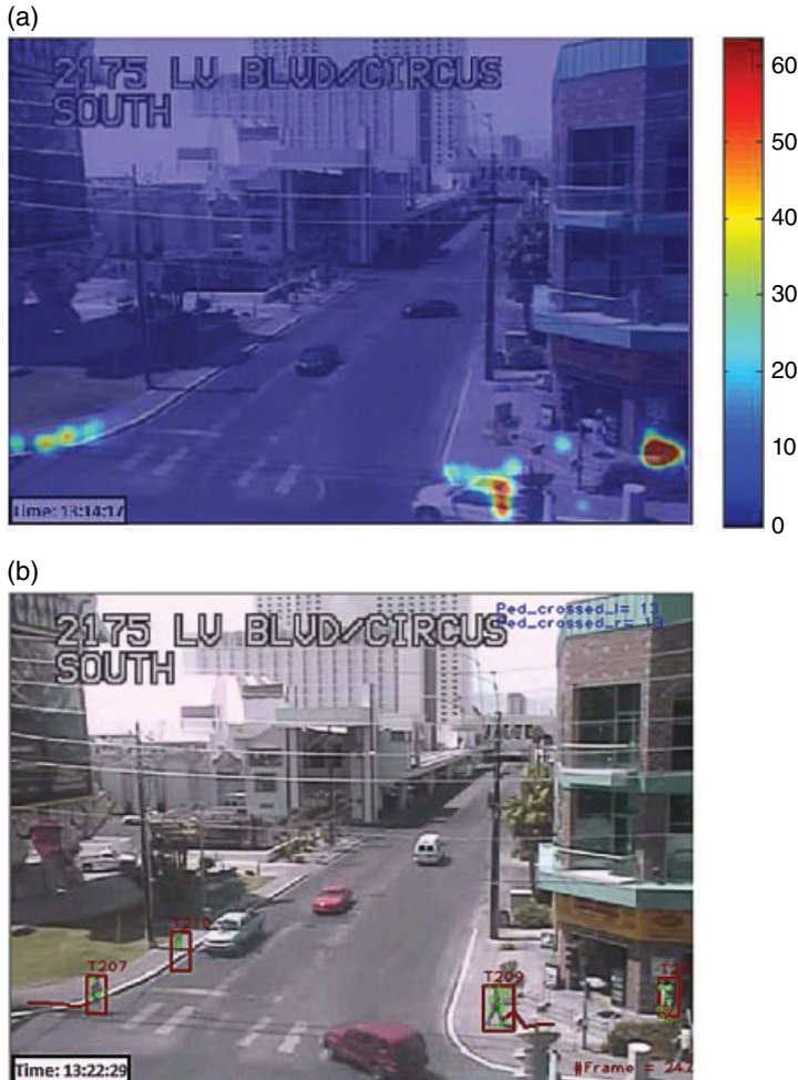
Figure 7.14 Waiting-time distribution and snapshot of tracking system which indicate a waiting pedestrian who talks with his phone for a long time period: (a) heatmap of waiting pedestrians and (b) snapshot of tracking system.
