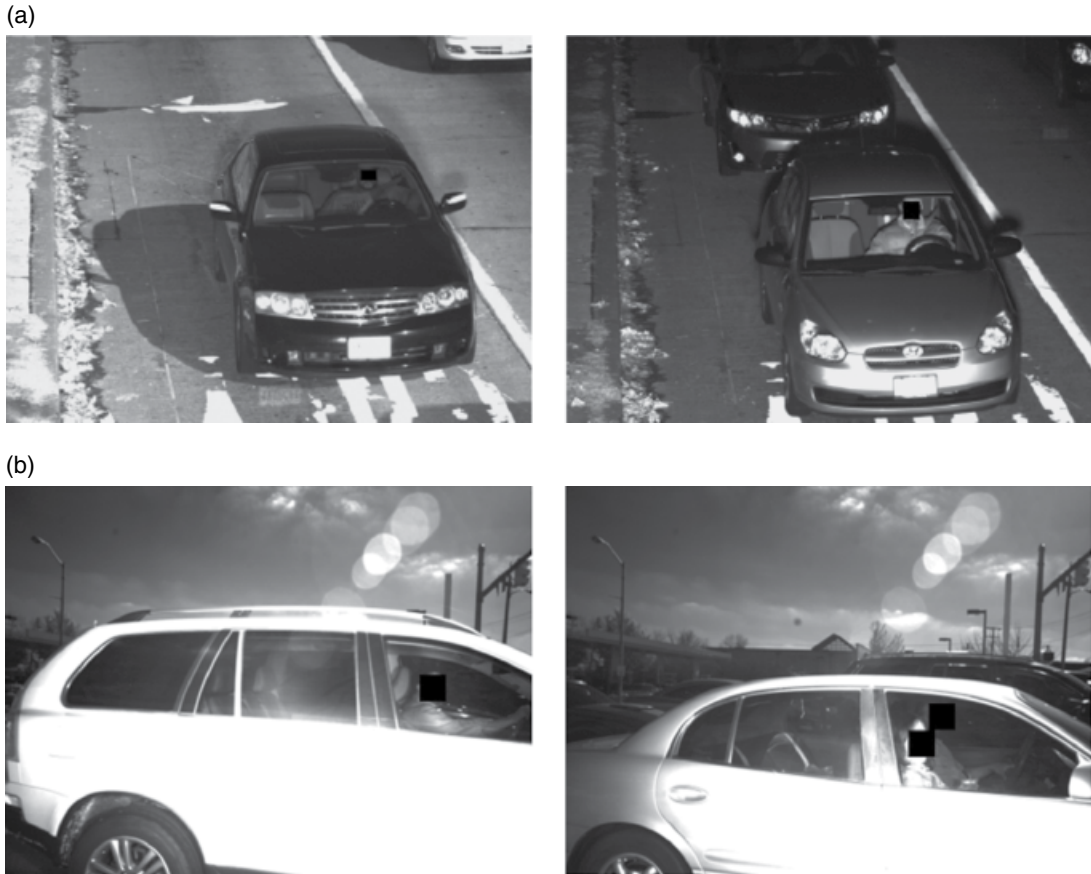
Figure 4.2 NIR images acquired by HOV/HOT lane front- and side-view cameras: (a) front-view images and (b) side-view images.
