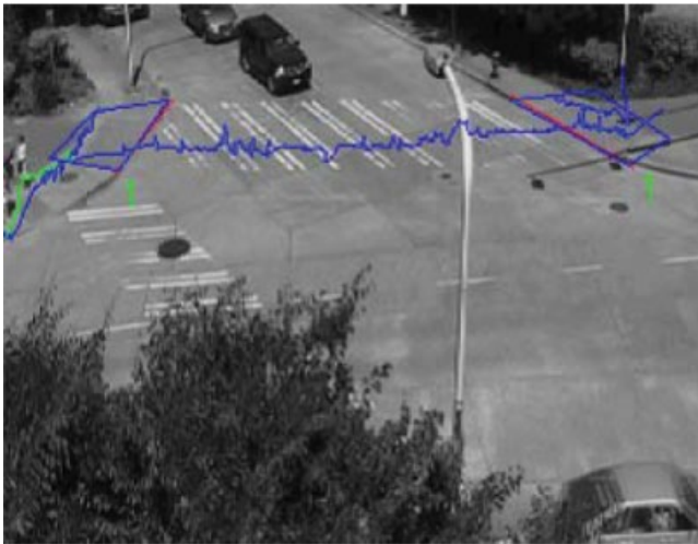
Figure 7.7 Complete crossing event [23] defined by traversal between waiting zones (trapezoids): (a) pedestrian crossing and (b) pedestrian data recorded. Source: Cho et al. [23]. Reproduced with permission of National Academy of Sciences.
