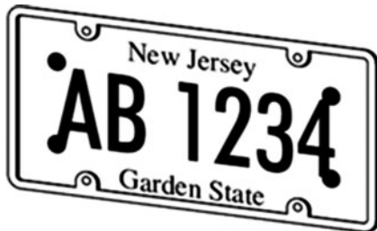
Figure 2.8 Cartoon of a coarsely cropped license plate ROI image output from the localization module.
