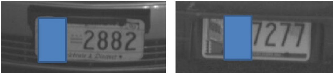
Figure 2.31 Partially redacted plate images with occlusion of the state name by license plate frames and car body features.
