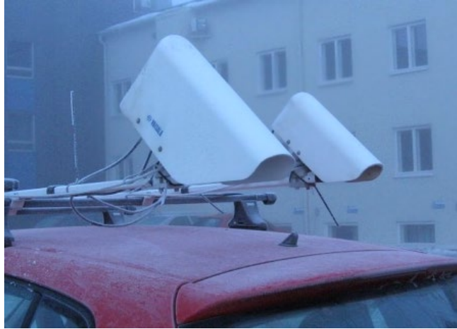
Figure 15.17 Vaisala's road weather sensors on the roof of the test vehicle.
