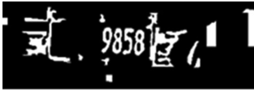
Figure 2.11 Remaining foreground blobs after morphological filtering and CCA.
