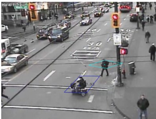
Figure 7.13 Crossing violation examples [36]. A spatial violation occurs when a pedestrian does not use the crosswalk. A temporal violation occurs when pedestrians cross the intersection during a “red-hand” phase. (a) Spatial violation and (b) temporal violation. Source: Zaki and Sayed [36]. Reproduced with permission of National Academy of Sciences.
