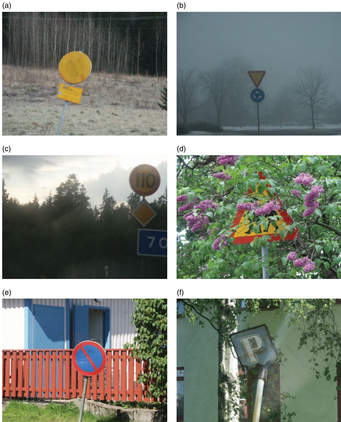
Figure 14.2 Potential challenges when working with traffic signs. (a) Faded sign, (b) bad weather condition, (c) bad lighting geometry, (d) obstacles in the scene, (e) similar background colour, (f) damaged sign, (g) distance related size, (h) motion blur, (i) reflection from sign board and (j) stickers.
