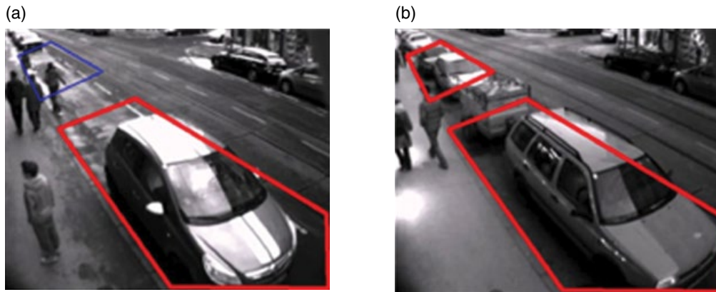
Figure 8.8 Typical detection results using the combined HOG–LBP detector. The disadvantage of site- and camera-specific training is offset by the excellent detection rate and very low false-positive rate of this approach. (a) Presence of pedestrians does not produce false alarms. (b) Cars' positive detections.
