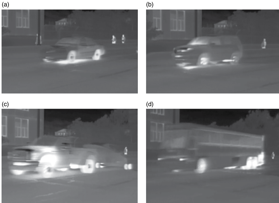
Figure 3.7 Example frames from a thermal camera for different vehicles: (a) small car, (b) SUV, (c) pickup truck, and (d) bus.
