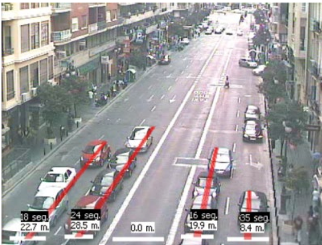
Figure 7.9 Detection-based queue length estimation uses nonmoving keypoints to estimate a queue line [28]. (a) Static corner points and (b) estimated queue length. Source: Albiol et al. [28]. Reproduced with permission of IEEE.
