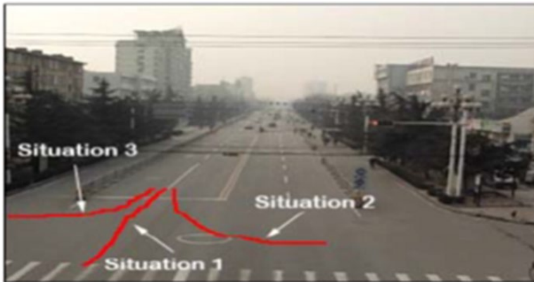
Figure 5.12 Three situations in the cross junction. The VLDs cannot distinguish right turns (situation 3) from the red light violations (situations 1 and 2). Source: Luo and Qin [51]. Reproduced with permission of IEEE.
