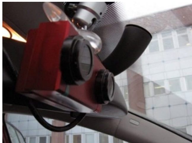
Figure 15.10 IcOR's stereo camera located inside the test vehicle.
