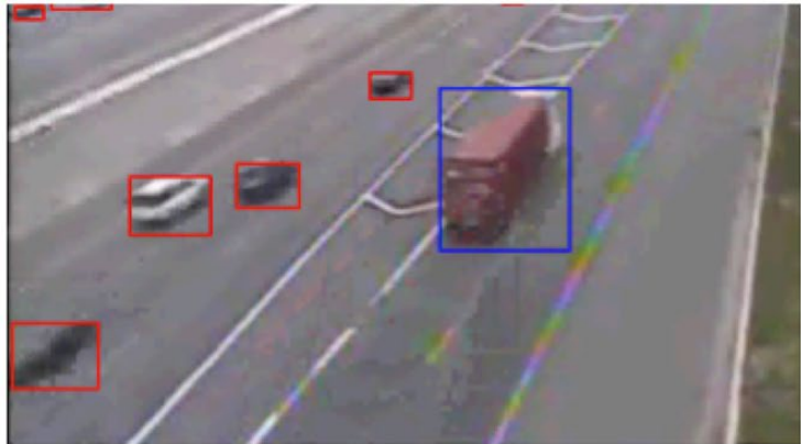
Figure 3.25 Screenshots for the classification of trucks (large boxes) and cars (small boxes) of the live videos from three cameras in different angles.
