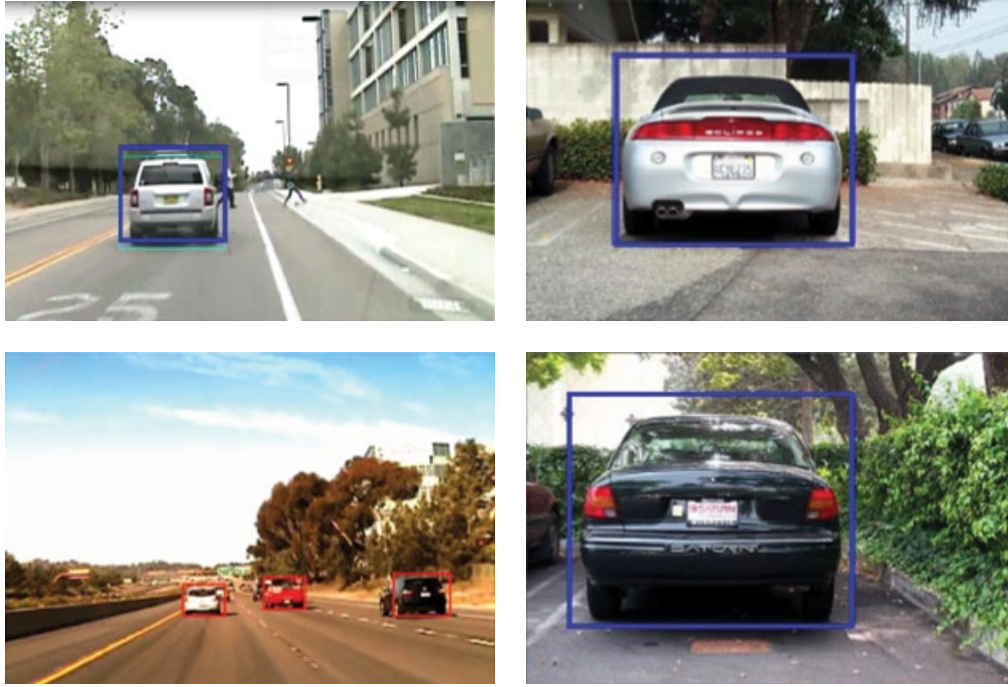
Figure 12.8 Sample results of vehicle detection in ELVIS.
