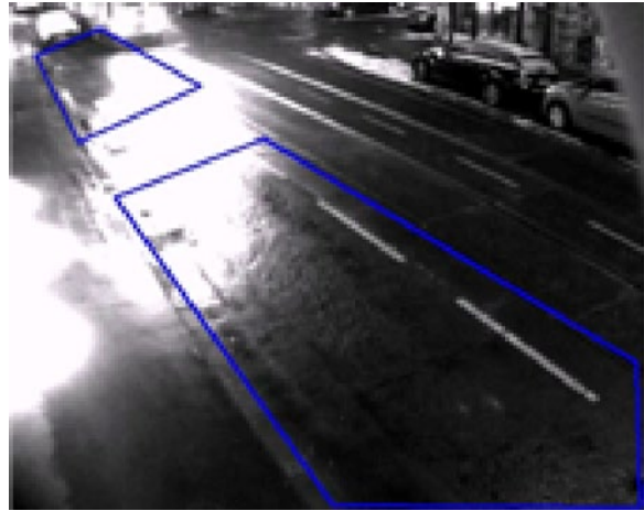
Figure 8.7 The loading zones which had to be monitored for the pilot project in the City of Vienna. This is a nighttime image of the two empty parking spaces. Harsh lighting situations, reflections, and adjacent heavy traffic complicate the detection task.
