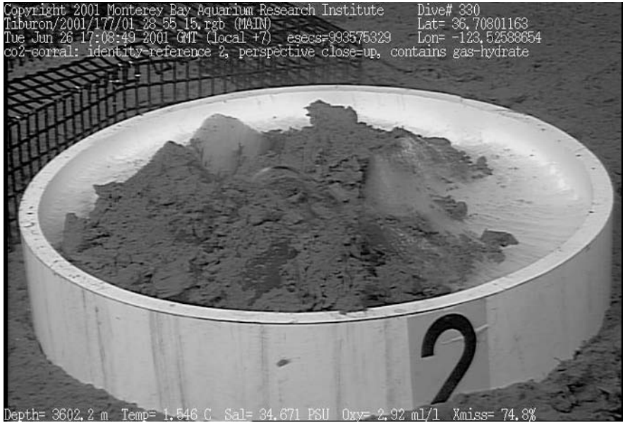
Figure 27.2. A “frost heave” of CO 2 hydrate on the sea floor at 3,600 m depth resulting from massive hydrate formation.
