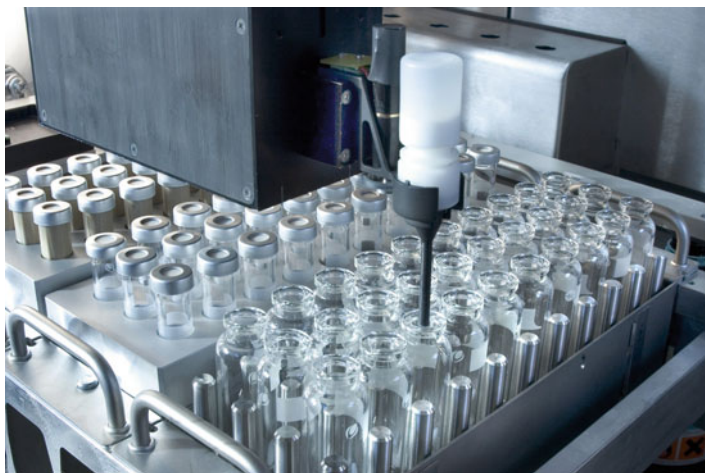
Fig. 13.5 Robot dispensing a powder. The “holder” is an analytical balance. Picture courtesy of Chemspeed Technologies AG
