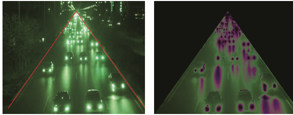
Fig. 3. (a) Pavement area; (b) Removal of headlights and strong reflections
