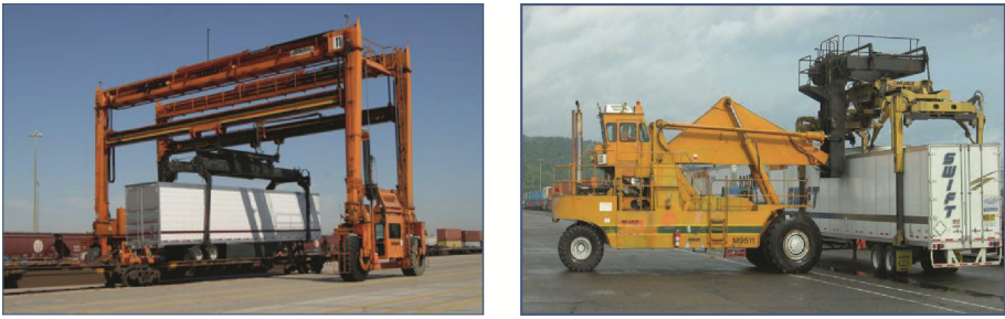
Fig. 1. The wrap-around crane and self-propelled crane of the van semi-trailer
