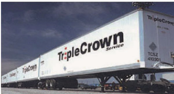
Fig. 2. Railway semi-trailer in USA
