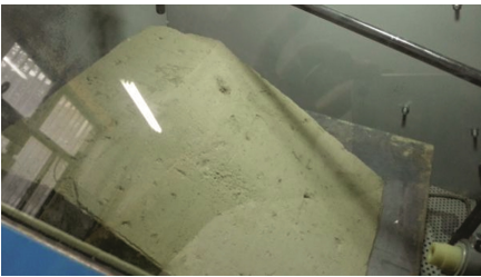
Fig. 1. Subgrade model is fed into sand blaster
