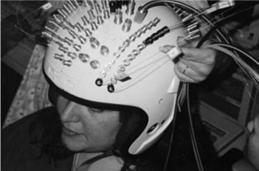
**FIGURE 9.2** The headgear (a modified motorcycle helmet) used to hold in place the source and detector fibers.
