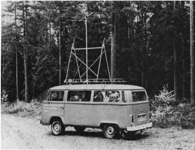
Fig. 1. Mobile tracking unit with the antenna elevated for operating. The antenna lowers from inside the vehicle to rest in the rack for driving.
