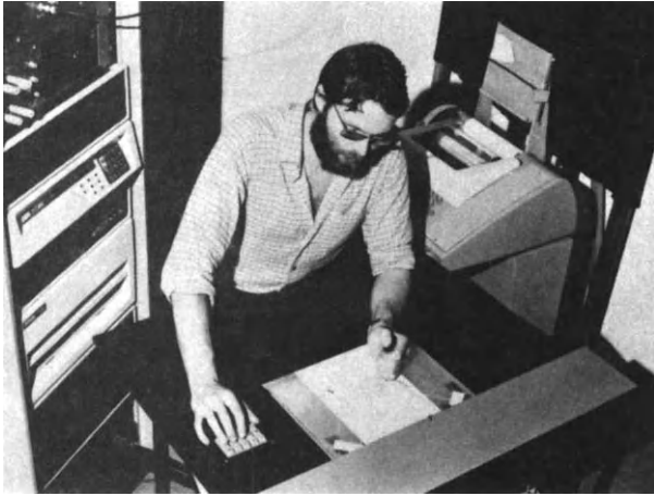
Fig. 5. An interactive x, y coordinate plotter, useful for the fast and efficient transcription of large numbers of radio fixes into scaled map coordinates ready for analysis. (a) Shows the plotting table in use while (b) shows the geometry underlying the plotting procedure.
