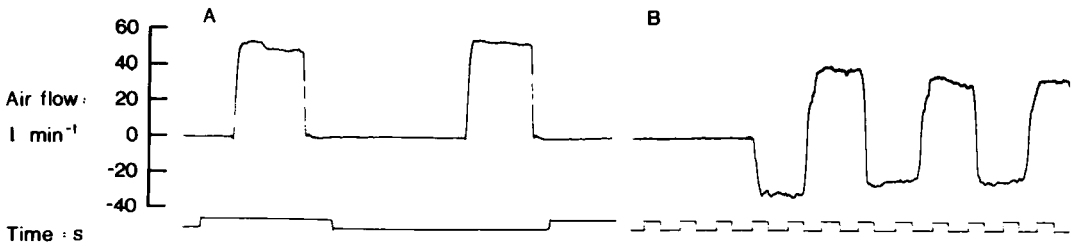
Fig. 5. Traces showing: (A) the response of the transducer to pulsed air flow; (B) respiration of a human, with the transducer used as an external flowmeter.
