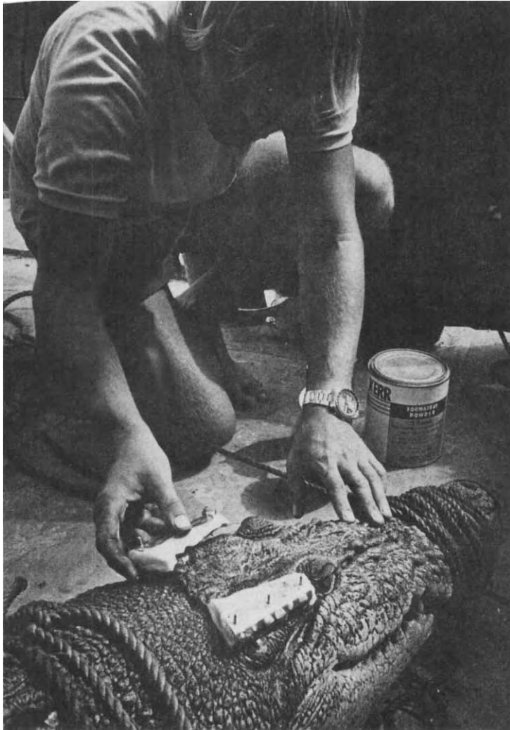
Fig. 7. Two moulds matching the bony protrusions above each ear take only a few minutes to form. The six bolts are used to secure an aluminum baseplate which supports the transmitter.
