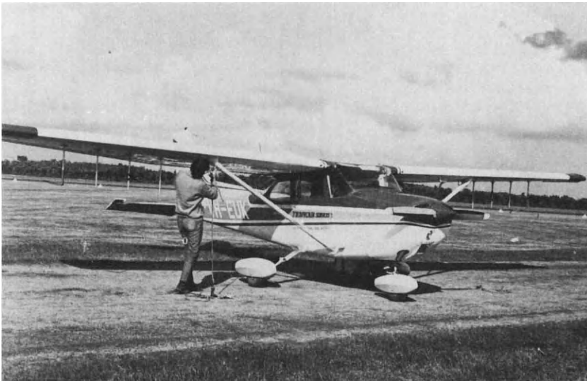
Fig. 3. End-fire monopole array mounted on Cessna 172 aircraft (from Whitehouse and Steven, 1977).
