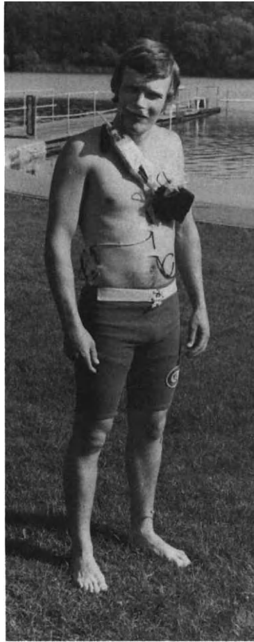
Fig. 7. Showing subject instrumentation used in the analysis of the spinal forces incurred during water-ski jumping.
