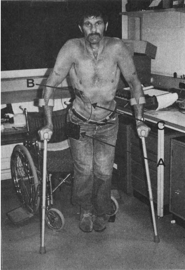
Fig. 5. Paraplegic Mr. G. L. standing with the aid of femoral nerve stimulation. (A) Rugged ABS box contains circuit of Fig. 3 and sufficient NiCd batteries for at least 12 h use between charges. (B) Araldite moulding containing six transmitters stuck to skin over receiver implant. (C) Cable and connectors between A and B.
