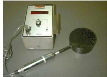
An exposure meter used in radiography.
