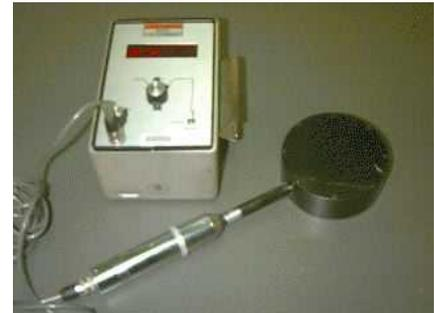
An exposure meter used in radiography.
