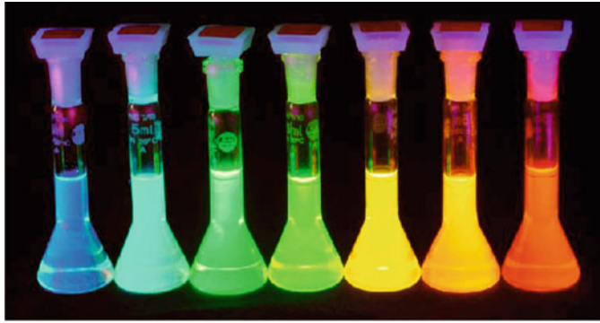
Fig. 7 Quantum dots sorted by size emitting light of different colors. Light-emitting core-shell Cd/Se/ZnS nanocrystals. D.V. talapin, A.L. Rogach, A. Kornowski, M. Haase, H. Weller. Highly Luminescent Monodisperse CdSe and CdSe/ZnS Nanocrystals synthesized in a Hexadecylamine-Trioctylphosphine Oxide-Trioctylphosphine Mixture. Nano Lett. 2001,1,207–211. With kind permission of Horst Weller Group, University of Hamburg
