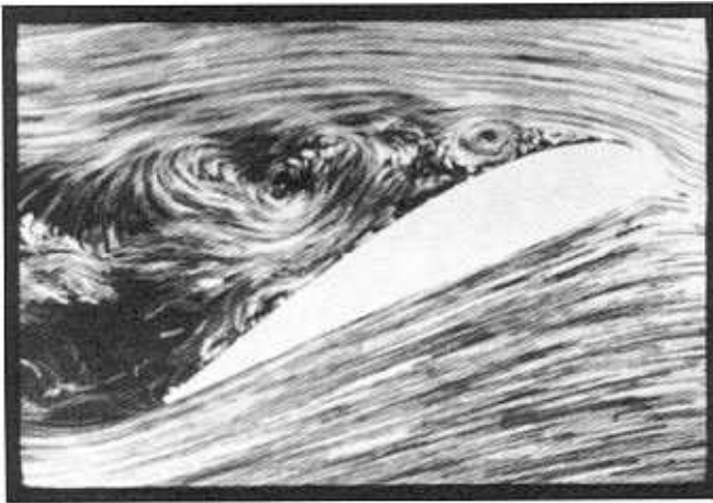
Figure 10b. Typical profile of airfoil at an angle of attack that gives fluids separation from the airfoil surface.
