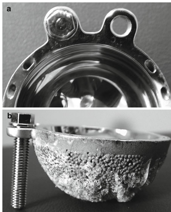
Fig. 24.7 Mickey Mouse ears/screw holes and screw in BHR dysplasia. (a) Front view and (b) side view
