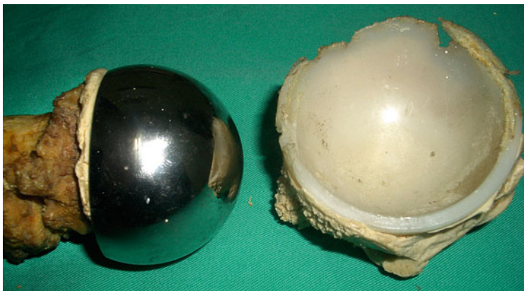
Fig. 22.3 Wagner resurfacing prosthesis removed at 18 months postsurgery. We can see the thin polyethylene liner, cause of the failure
