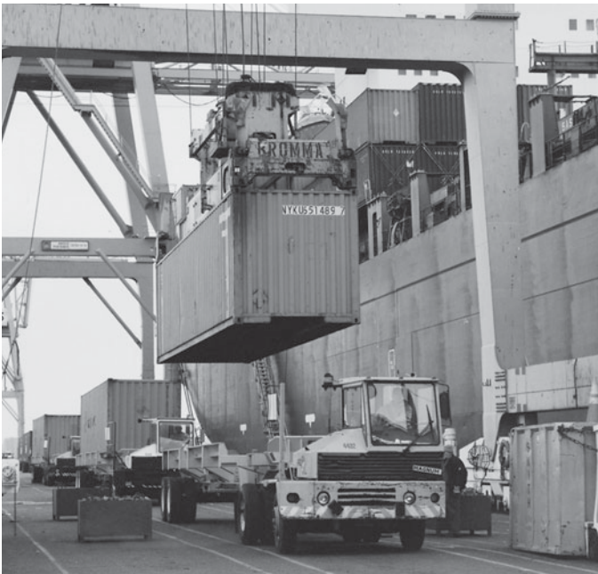
FIGURE 9.13 Container cargo handling at the Maersk Line Terminal, Port Newark, New Jersey. Containerization has greatly improved the operation, management, and logistics of oceangoing freight. The container revolution has impacted more than conventional shipping and international trade. Newly designed cellular vessels have much faster turnaround time in port and have improved cargo-handling productivity at ports. Moreover, the interface between water and land transportation has expanded. The new container trains have enhanced the economy and scale of rail transportation.
