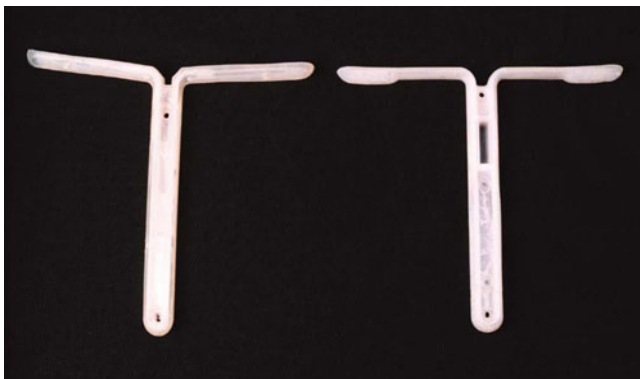
Fig. 11.5 The original CIDR-B ( left ) and the optimized version named the CIDR 1380 Cattle Insert ( right )
