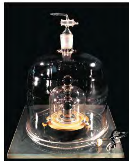
1.4 The international standard kilogram is the metal object carefully enclosed within these nested glass containers.
