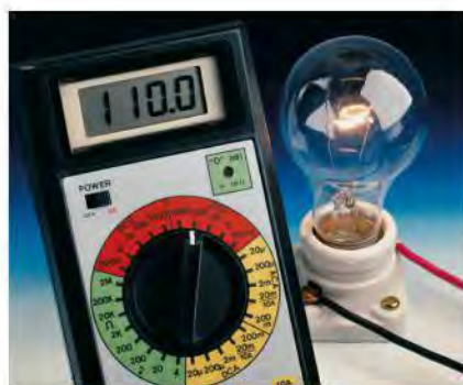
26.18 This digital multimeter can be used as a voltmeter (red arc), ammeter (yellow arc), or ohmmeter (green arc).
