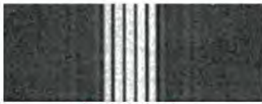
For d = 4a , every fourth interference maximum at the sides ( m_i = \pm 4, \pm 8, \dots ) is missing.
