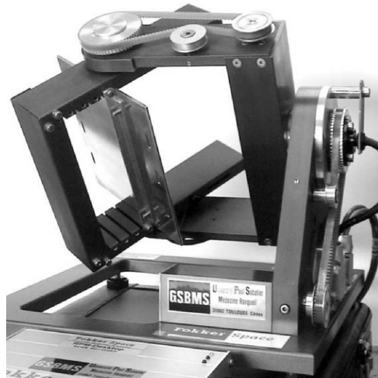
Figure 3-07. The three-dimensional clinostat, also called Random Positioning Machine (RPM), creates a condition in which the weight vector is continually reoriented in all directions. Photo courtesy of Gilbert Gasset, GSBMS, Toulouse.
