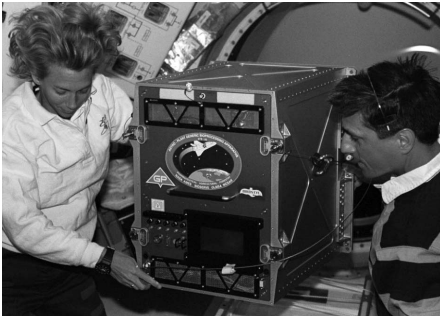
Figure 8-02. The Generic Bioprocessing Apparatus on board the Spacelab Science Module in the Space Shuttle Columbia (STS-94), shortly after arriving on orbit. The bioprocessing reactions involved sequential mixing of fluids for phase processing, incubation, optical monitoring, and temperature storage. This facility could host up to 132 individual experiments. Experiments included studies of how collagen fibers could be used more effectively as artificial skin or blood vessels, how the assembly of liposomes and virus capsids could be used to target a drug to specific tumors, or how mineralization occurs and influences the embryonic bone tissue of rodents. Photo courtesy of NASA.
