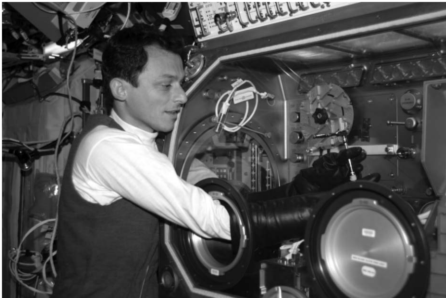
Figure 3-23. The glovebox provides a sealed work area where crewmembers can perform experimental procedures such as subsampling cultures, fixating preparations, fluid chemical handling, and harvesting plants. Photo courtesy of NASA.
