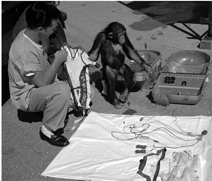
Figure 2-03. This photograph shows the biosensors used for monitoring the physiological parameters of monkeys during spaceflight. Photo courtesy of NASA.
