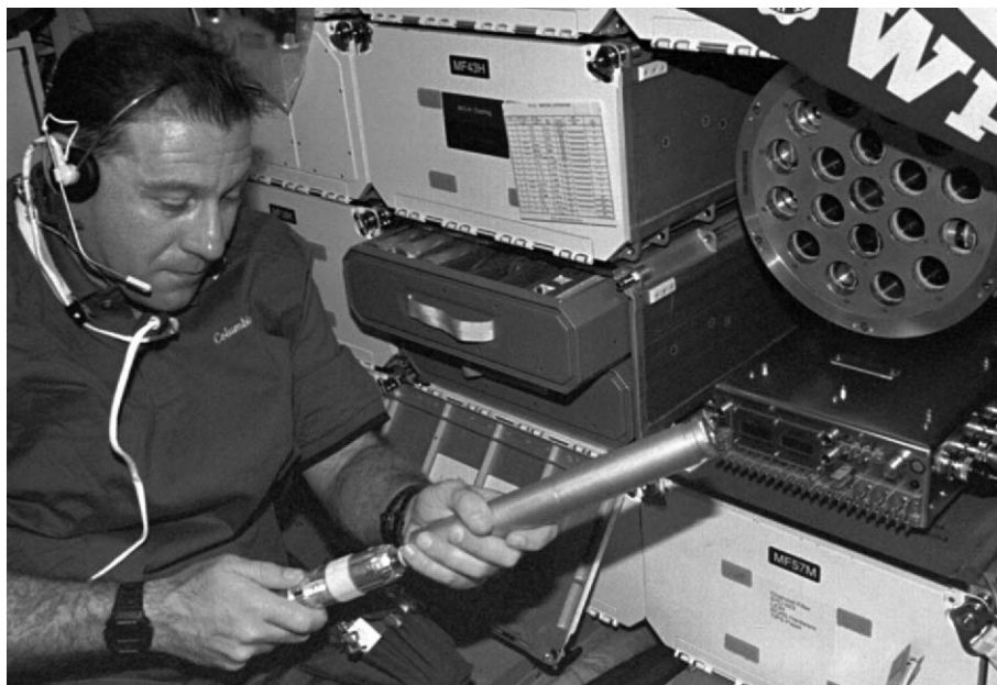
Figure 8-12. Dr. Albert Sacco flew as a Payload Specialist operating his own zeolite crystal growth experiment onboard STS-73 in 1995. On this photograph, he is inspecting a crystal in a cylindrical autoclave on the middeck of Space Shuttle Columbia. Photo courtesy of NASA.
