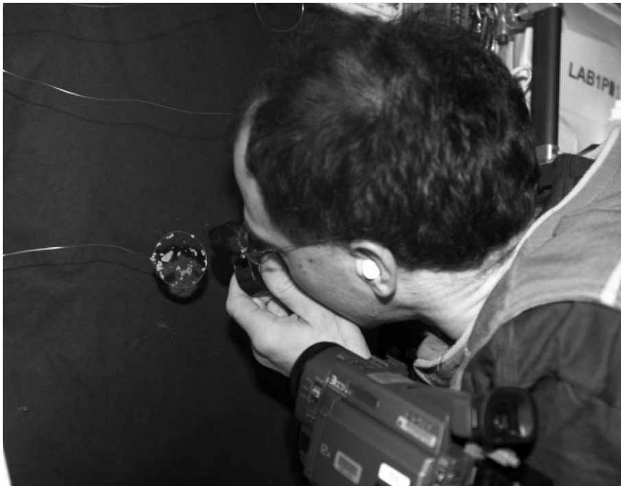
Figure 8-10. Astronaut Donald R. Pettit, during his spare time on board the ISS, built a small laboratory to experiment and observe the behavior of fluids and crystals in microgravity. This activity used simple materials that would not impact the programmatic supplies and was dubbed "Saturday Morning Science". In this photograph, he is shown looking closely at a water bubble within a 50-millimeter metal loop. Photo courtesy of NASA. Source: http://spaceflight.nasa.gov/station/crew/exp6/spacechronicles18.html
