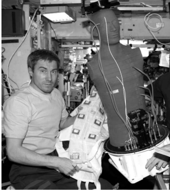
Figure 7-19. ISS Cosmonaut Sergei K. Krikalev holds the anthropomorphic phantom Matroshka, a human-torso-like device, after its retrieval from the exterior of the ISS during a spacewalk, for return to Earth. The experiment is designed to better understand the exposure of astronauts, including those making spacewalks, to radiation. Photo courtesy of NASA.
