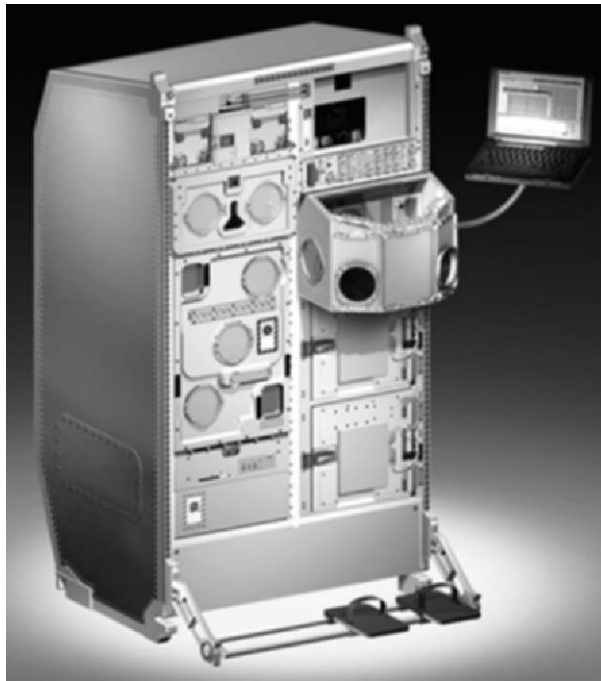
Figure 4-02. Within the Biolab facility, experiments on board the International Space Station can be incubated, stored at cool or cold temperatures, microscopically or photometrically analysed and freshly prepared, if required, allowing most of these features without crew interaction, but with telescience capability. Source ESA.
