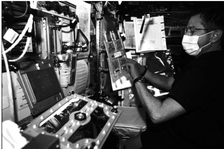
Figure 8-03. Astronaut Frank L. Culbertson works at the NASA bioreactor rotating wall vessel in the Destiny laboratory on board the ISS. The bioreactor comprises four incubation/refrigeration chambers. Every 7 to 21 days (depending on growth rates), an astronaut uses a shrouded syringe and the bags' needleless injection ports to transfer a few cells to a fresh media bag, and to introduce a fixative so that the cells may be studied after flight. The design also lets the crew sample the media to measure glucose, gas, and pH levels, and to inspect cells with a microscope. Photo courtesy of NASA.
