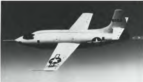
16.37 The first supersonic airplane, the Bell X-1, was shaped much like a 50-caliber bullet—which was known to be able to travel faster than sound.
