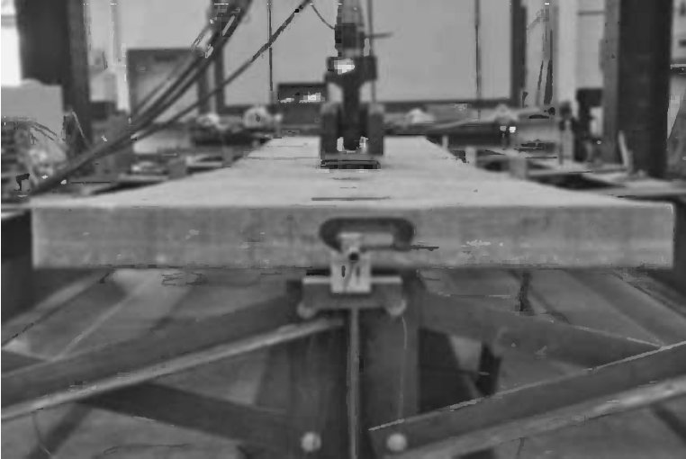
FIGURE 5.19 T-section prior to failure.
