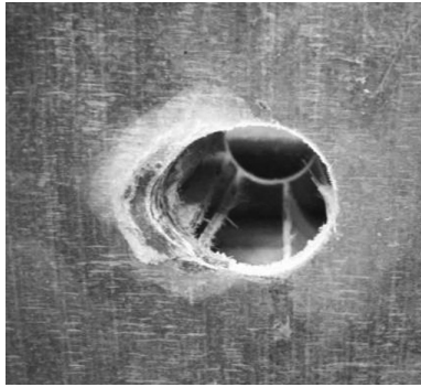
FIGURE 4.7 Delamination of bottom FRP facesheet.
