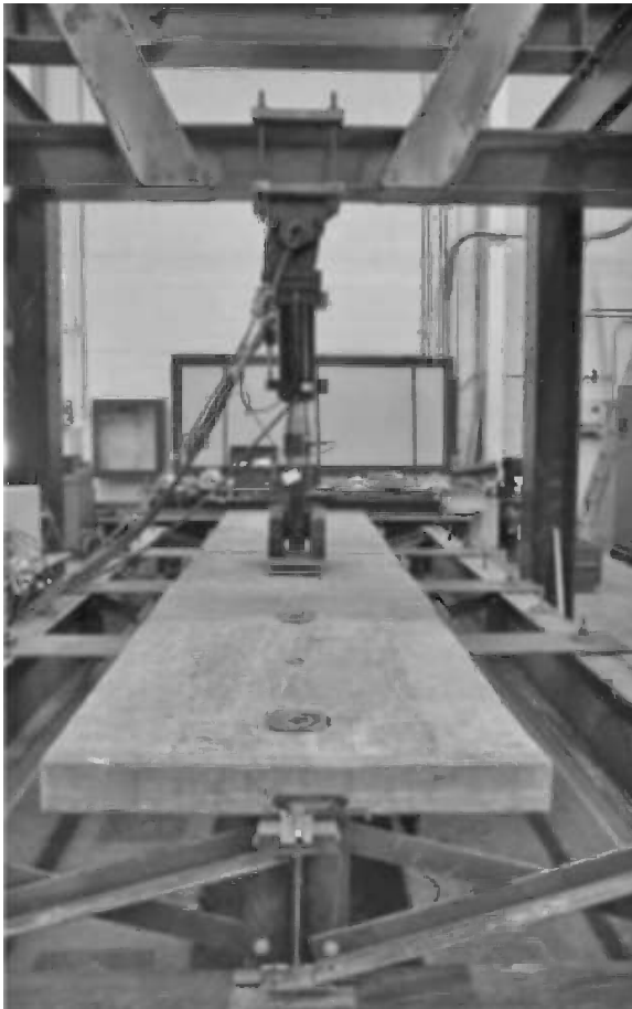
FIGURE 5.6 Installations of shear connection to FRP decks.
