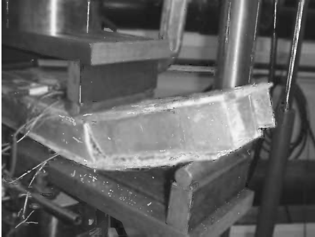
FIGURE 3.50 Shear crushing of the core.
