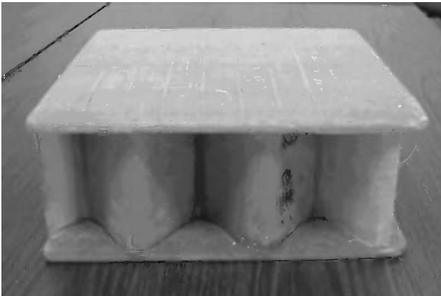
FIGURE 2.1 FRP honeycomb sandwich panel.
