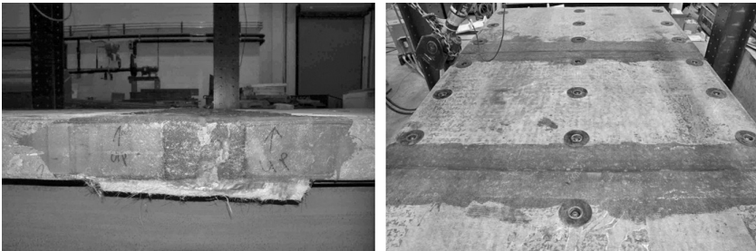
FIGURE 5.4 Tongue-and-groove connection with FRP sheet covered.
