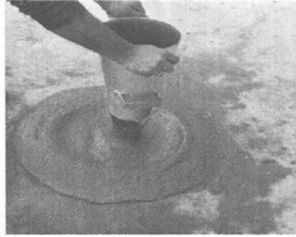
FIG. 2—Flowability measurements using an inverted slump cone.
