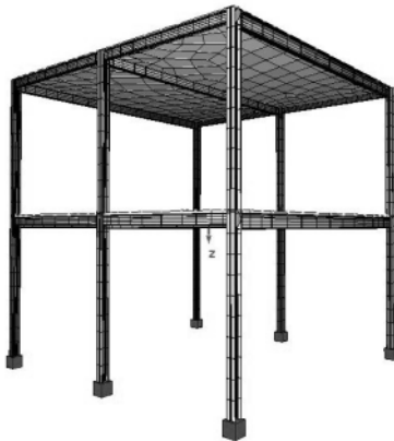
Figure 2.4 – Structural model with two-dimensional elements
