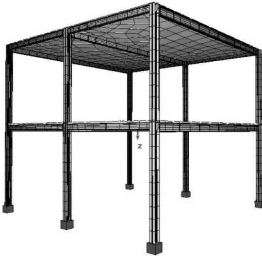
Figure 2.20 – Beam and shell structural model
