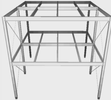
Figure 2.42 – Structural steel model (neglecting the slab)
