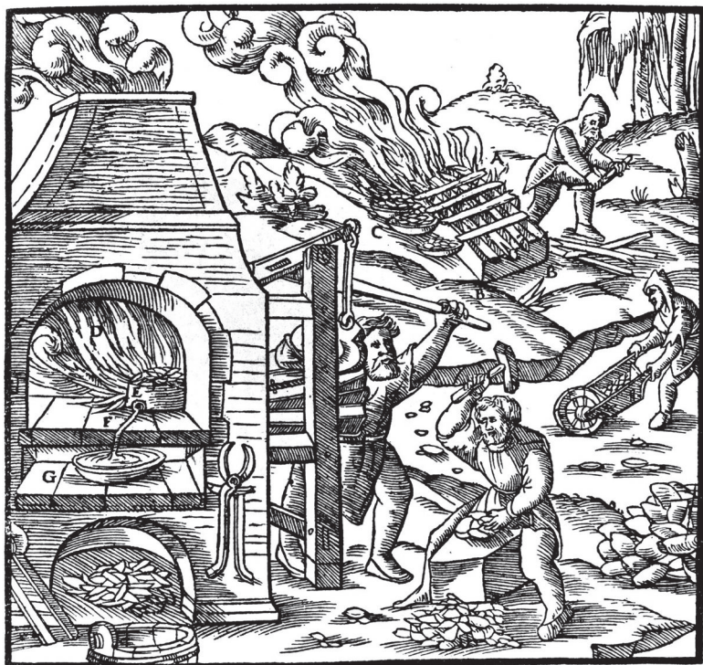
A—WOOD. B—BRICKS. C—PANS. D—FURNACE. E—CRUCIBLE. F—PIPE. G—DIPPING-POT.
