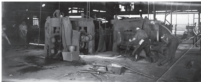
FIGURE 4.5 A puddler and his helper remove a 150-pound, near-molten ball of wrought iron from a puddling furnace, Youngstown, Ohio, 1920s. Photographer unknown. Source: https://thatdevilhistory.wordpress.com/2014/01
