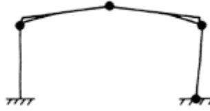
Figure 11.11 Basic collapse mechanism (Mode 1) for haunched portal.
