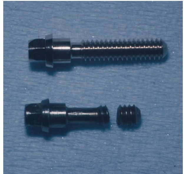
Figure 16.11 The lower screw is a retrieved fractured Branemark abutment screw, compared with an intact screw above it. The fractured screw was removed from the case illustrated in Figure 16.12.
