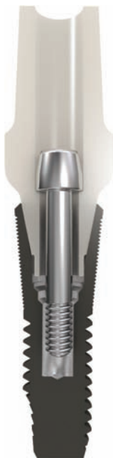
Figure 1.13 Section through a single tooth Astra Tech implant with a zirconium abutment, connected via an internal connection and titanium abutment screw.
