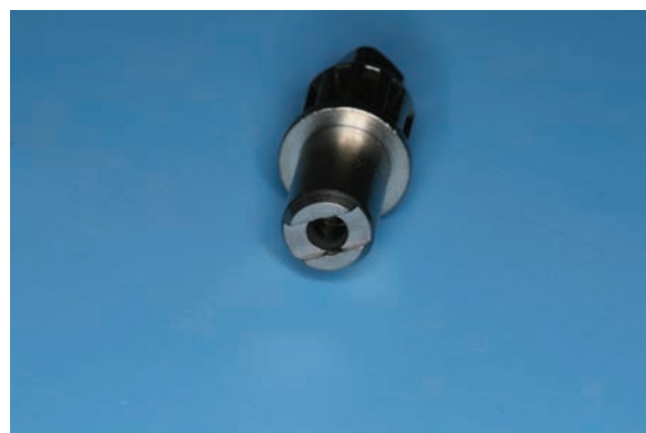
Figure 15.15 Astra ball abutment driver. This is used to insert the abutment into the implant. The drive is attached to a torque wrench and the ball abutment is torqued to 20 or 25 Ncm according to manufacturer's guidance.
