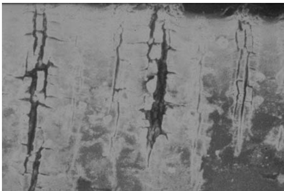
Fig. 4 Scanning electron micrograph of the conductor-contacting inner surface of a lead's insulation showing MIO degradation where the tubing contacted the metal coils
