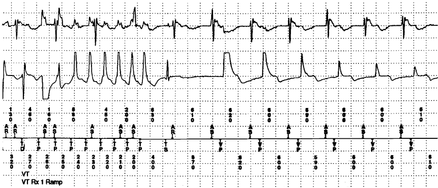
FIGURE 6.32c. From top to bottom: atrial electrogram, ventricular electrogram, and marker channel. Markers: AR = atrial refractory sense; AS = atrial sensing; TS = tachycardia sensing; TD = tachycardia detected; TP = tachycardia pacing; VP = ventricular pace; VS = ventricular sense.
